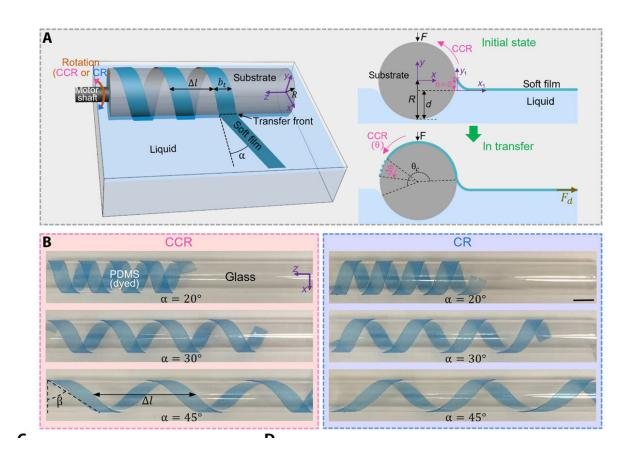
Elastocapillary rolling transfer weaves soft film to spatial helical structure on curved substrates. Credit: *Science Advances* (2023). DOI: 10.1126/sciadv.adh9232
