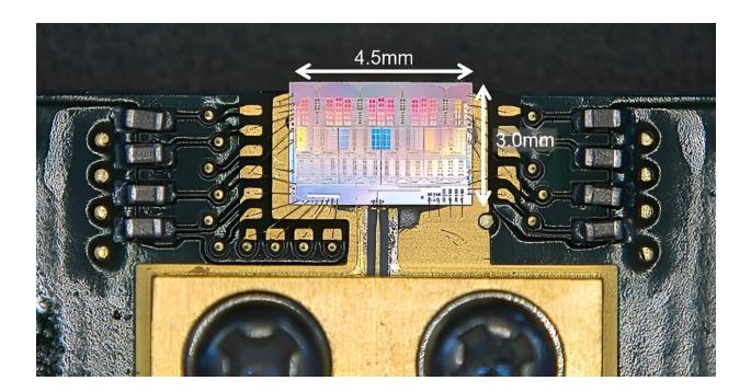
Development of a 150 GHz transmitter IC chip and supporting technologies. Credit: NEC Corporation
