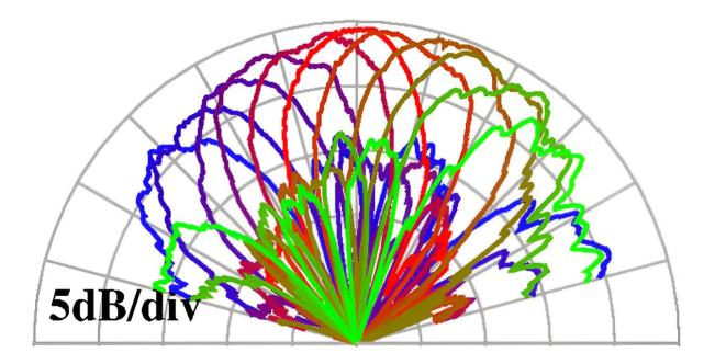
4-channel antenna radiation pattern measurement results (150GHz). Credit: NEC Corporation
