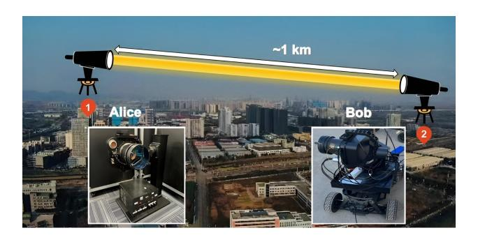
A free-space optical communication experiment involves a pair of FSO devices with one ("Alice") fixed on the top floor of a building, while the other ("Bob") is loaded on a radio-controlled electric vehicle so that it can move around to vary the distance of the FSO link nodes. Credit: Liu, Zhang, et al., doi 10.1117/1.APN.2.6.065001.
