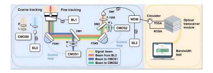
FSO device design. L, lens; IF, interference filter; DM, dichroic mirror; WDM, wavelength division multiplexer; TOSA, transmitter optical subassembly module; ROSA, receiver optical subassembly module; CMOS, complementary metal oxide semiconductor; BL, beacon laser; and FSM, fast steering mirror system. Credit: Liu, Zhang, et al., doi 10.1117/1.APN.2.6.065001.
