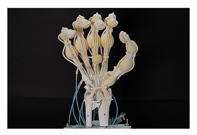
Researchers produced a functional, tendon-driven robotic hand that has 19 independently actuatable tendons, soft fingers with sensor pads, and rigid, load-bearing bones. Credit: Wojciech Matusik, Robert Katzschmann, Thomas Buchner, et al
