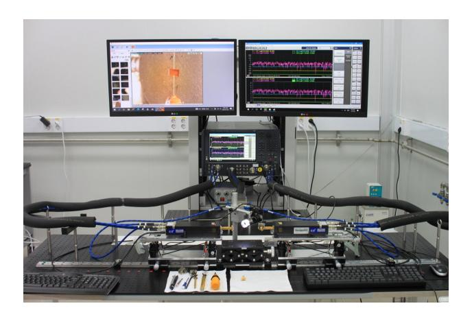
Electromagnetic impedance measurement system developed by KRISS researchers. Credit: Korea Research Institute of Standards and Science (KRISS)
